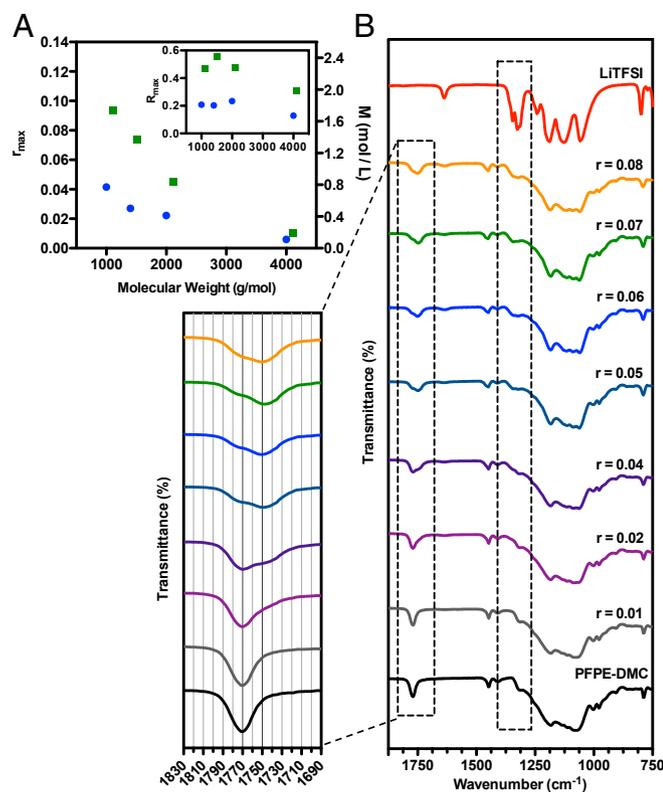
**Fig. 3.** Characterization of LiTFSI loading in PFPE electrolytes. (A) Maximum LiTFSI loading in PFPE-diols (blue) and PFPE-DMCs (green) expressed in  $r_{max}$ , the molar ratio of  $\text{Li}^+$  ions to repeating fluoroether units and molarity, and in  $R_{max}$  (Inset), the molar ratio of  $\text{Li}^+$  ions to end group functionalities, as a function of molecular weight. (B) IR spectra of PFPE<sub>1000</sub>-DMC/LiTFSI blends at different concentrations.
