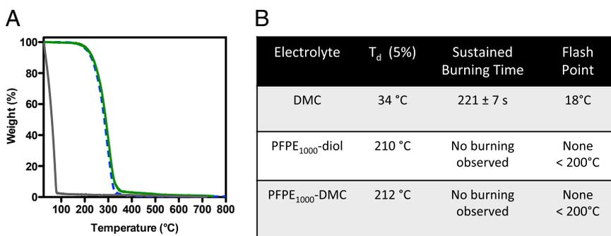
**Fig. 2.** Thermal stability and flammability of PFPEs. (A) TG curves for thermal decompositions of DMC (solid gray), PFPE<sub>1000</sub>-diols (dashed blue), and PFPE<sub>1000</sub>-DMCs (solid green). (B) Corresponding decomposition temperature (5%), sustained burning characteristics, and flash points of these materials.
