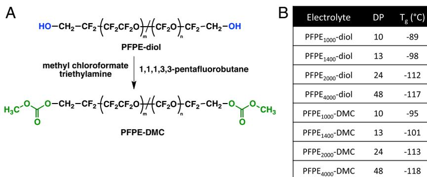
**Fig. 1.** PFPE oligomers as Li-ion electrolytes. (A) Chemical reaction scheme describing the synthesis of PFPE-DMC from PFPE-diol. (B) PFPE-diol and PFPE-DMC electrolytes with corresponding degrees of polymerization and glass transition temperatures.
