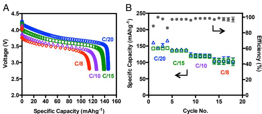
**Fig. 5.** Cyclability of Li/PFPE<sub>1000</sub>-DMC-LiTFSI/LiNMC cells. (A) Discharge profiles obtained at 30 °C at different rates from C/20 to C/8 for a typical prototype Li/PFPE<sub>1000</sub>-DMC-LiTFSI/LiNMC. (B) Cycle performance of battery prototypes showing discharge (green □) and charge (blue △) capacities, as well as overall efficiencies (gray ●).
