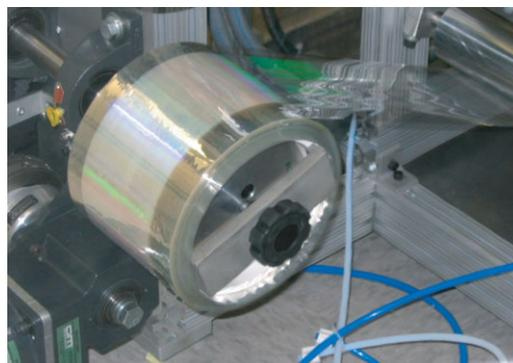
**FIGURE 2** | Continuous thin mold manufacturing for the PRINT process. Patterned surface can be seen in green. (Reprinted with permission from Ref 71. Liquidia Technologies.).
